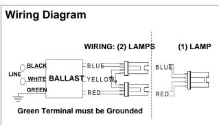
The wiring diagram that appears above is for the lamp type denoted by the asterisk  $(\ensuremath{^*})$
