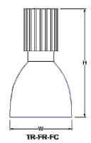
**FINISH-**Five stage pretreatment process, coated with a lead free TGI C polyester powder coat finish. White is standard inside reflectors, Except #49-Galvanized, #62-Anodized Bronze and #63-Iron Rust, Unless specified. Custom colors and Marine are available upon request.
