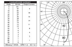
50% Beam width = 36.6° (ft.) Footcandles Beam Distance (ft.) Beam Dia. (ft.) 0.5 404.0 91 1.0 101.0 1.5 44.9 2.0 25.3 2.5 16.2 3.0 11.2 3.5 8.2 4.0 6.3 4.5 5.0 5.0 4.0 5.5 3.3 6.0 2.8
