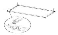
FIK: Designed to be used with any grid type recessed luminaire in ceiling requiring flanges. May be nailed to framing for purpose of trimming out the ceiling opening not to be used for support of lumimaire. If this method of installing FIK is used luminaire must be supported by #12 ga. mild steel wire by others.
