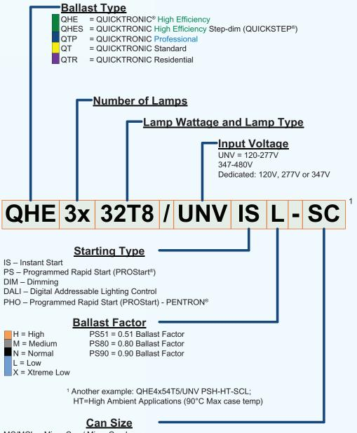
MC/MCL = Micro Can / Micro Can Long SC/SCL = Small Can / Small Can Long TC/TCL = Thin Can / Thin Can Long W = Wide Can DM = Dual Mount DM PEM = Dual Mount with PEM studs F = "F" Enclosure B = "B" Enclosure Blank = Standard Can
