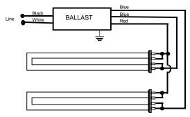
Note: For one lamp application, cap one blue lead, insulate to 600 volts
