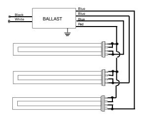
Note: For two lamp application, cap one blue lead, insulate to 600 volts
